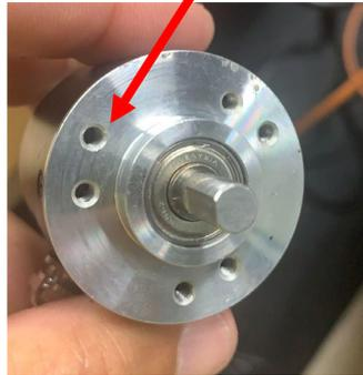
The encoder mounts to its bracket with 1 flathead screw (provided).
