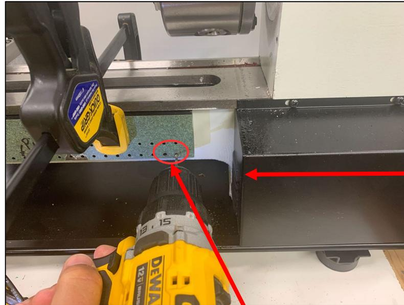
Tap the holes with a 3mm x .5 Metric tap. If you use a spiral tap, you can use a drill to tap the holes.
