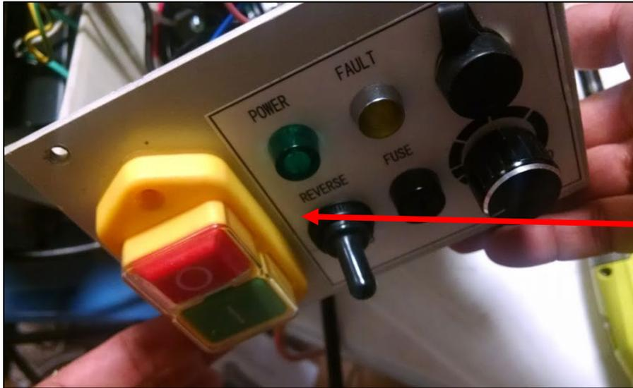
To prepare for the spindle wiring modifications to the lathe, first unplug the power cable to the lathe. We will need to bypass the on-off switch and the control wiring within the spindle control box. Remove the 4 philips screws holding the box to the lathe.
