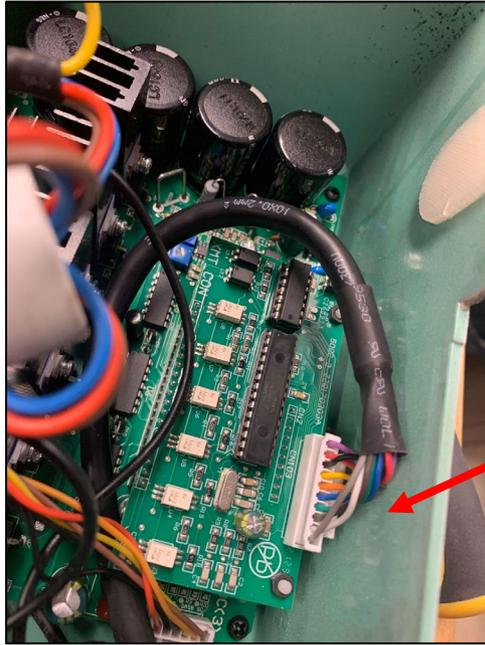
Remove the White connector the controls the speed of the motor. Note the screwdriver below
