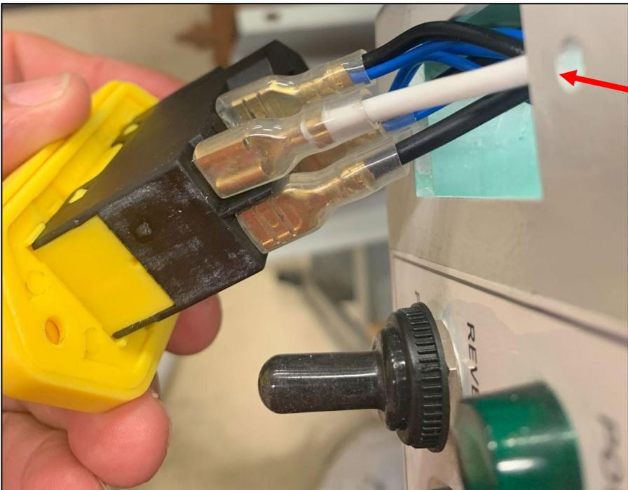
Note the color and positions of the wiring to the switch—yours may be different. Note the switch orientation—yours may be different, but the switches themselves are all the same.
