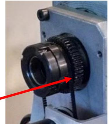
The encoder mounts to the headstock side of the lathe. It is driven by a 1:1 pulley system mounted to the lathe spindle.
