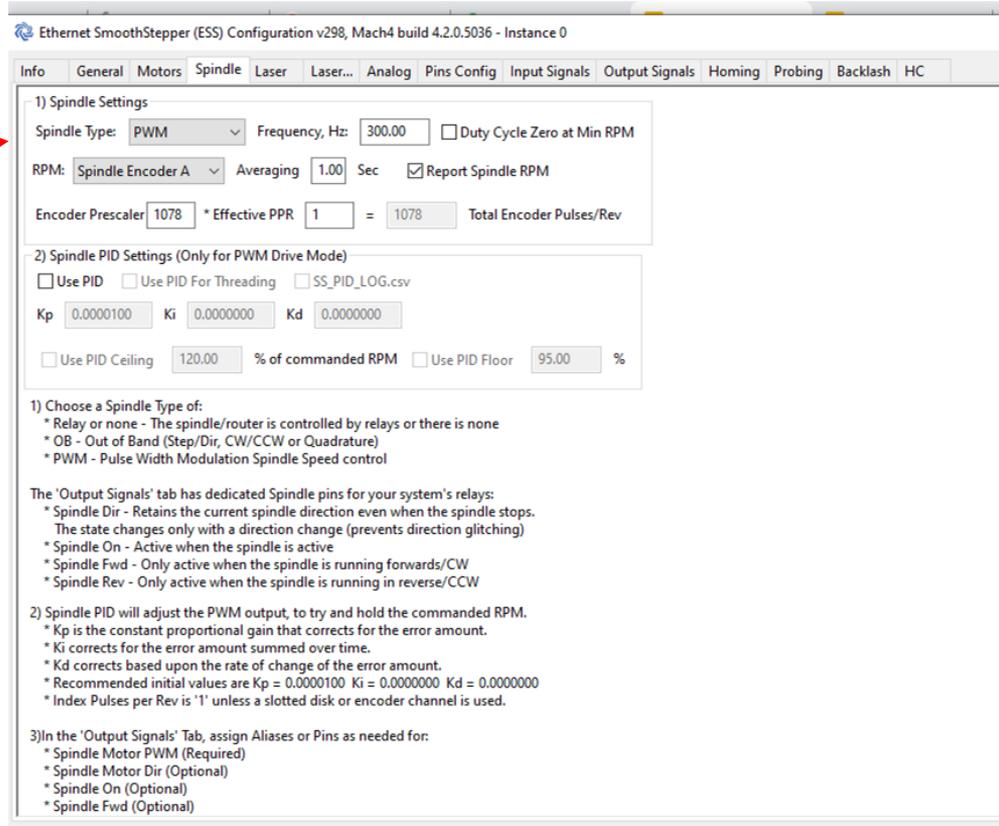
Ethernet SmoothStepper (ESS) Configuration v298, Mach4 build 4.2.0.5036 - Instance 0
