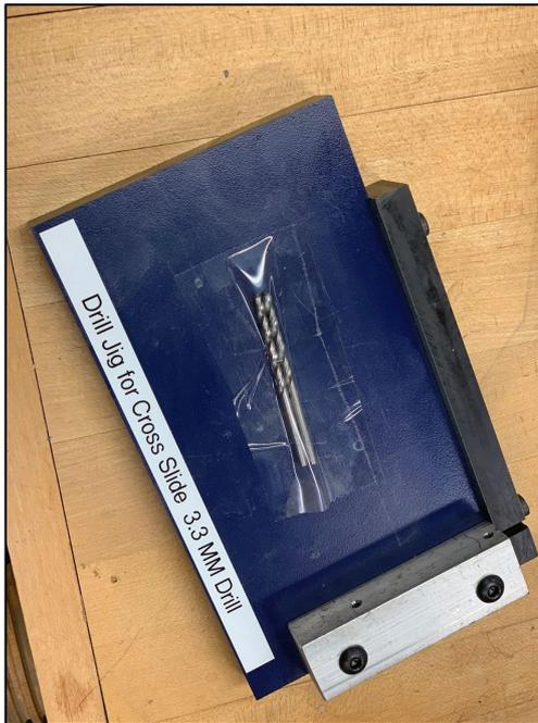
The cross slide will need to be drilled and tapped in 2 places for mounting the X-axis ballnut mounting bracket. The fixture shown on the left will assist in the accurate location of these holes. The cross slide will be drilled at 3.3 mm diameter for M4 x .7mm tapped holes.
