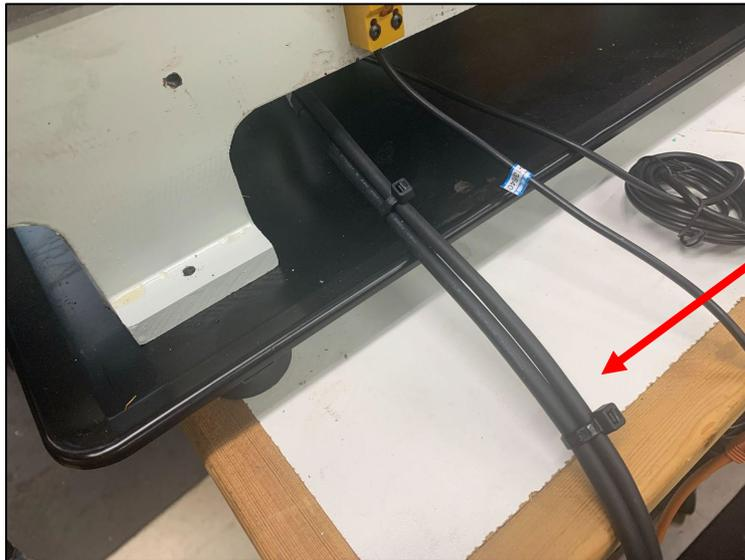
It's a good idea to tie the stepper motor cables together with zip-ties
