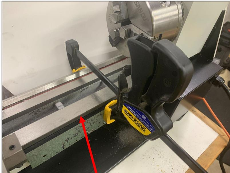
Align drill fixture with the "Datum" against the bottom side of the Z travel (ways)
